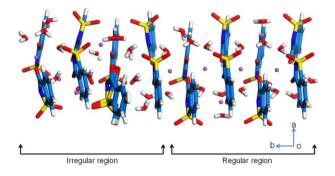
**Fig. 1.** Asymmetric unit of sodium saccharin dihydrate. The irregular regions are on the left side and the regular regions on the right side. Nanoindentation is performed on the (001) face in other words down the plane of the page.
