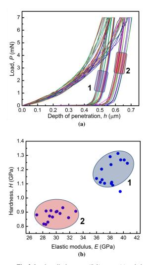
**Fig. 2.** Load *vs.* displacement (*P-h*) curves (a) and plot of hardness (*H*) *vs.* elastic modulus (*E*) of sodium saccharin dihydrate crystals (b) obtained with indentation normal to the (001) face
