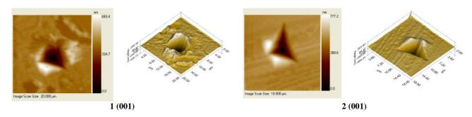
Fig. 3. AFM images of indent obtained on (001) after indentation
